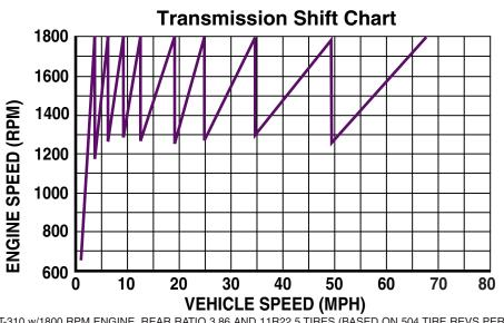
T-310 w/1800 RPM ENGINE, REAR RATIO 3.86 AND 11R22.5 TIRES (BASED ON 504 TIRE REVS PER MILE)
