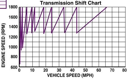
T-310MLR w/1800 RPM ENGINE, REAR RATIO 4.64 AND 11R22.5 TIRES (BASED ON 498 TIRE REVS PER MILE)
