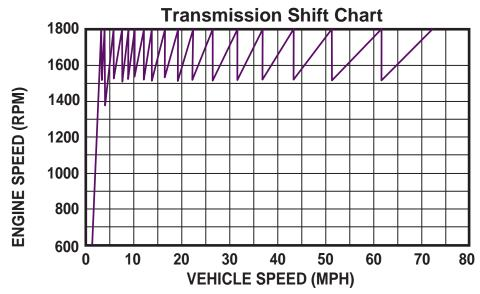
T-318 w/1800 RPM ENGINE, REAR RATIO 4.17 AND 11R22.5 TIRES (BASED ON 504 TIRE REVS PER MILE)
