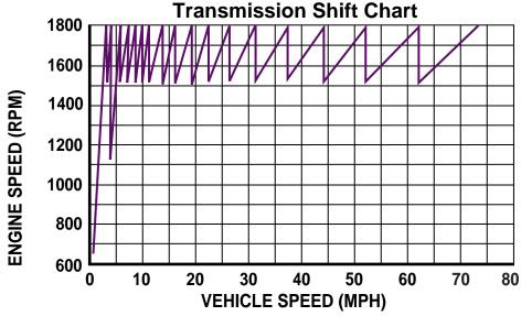
T-318LR w/1800 RPM ENGINE, REAR RATIO 4.17 AND 11R22.5 TIRES (BASED ON 504 TIRE REVS PER MILE)
