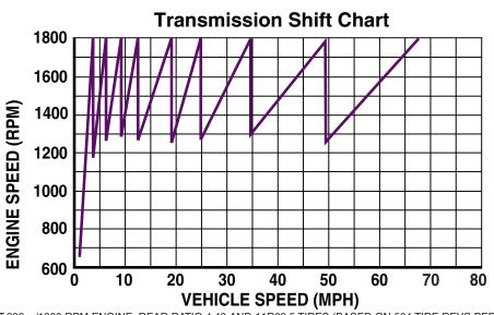
T-309 w/1800 RPM ENGINE, REAR RATIO 4.42 AND 11R22.5 TIRES (BASED ON 504 TIRE REVS PER MILE)
